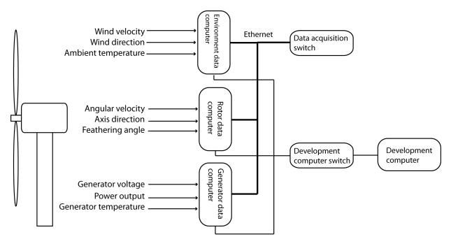
To record the data and timestamps, you connect the sensors to a set of data acquisition target computers. You interconnect the data acquisition computers through an Ethernet network and a switch that supports the PTP protocol (a PTP transparent clock or boundary clock). To access the data and timestamps, you connect the target computers to a development computer through another Ethernet network and switch. On the development computer, you run MATLAB to do the data analysis, including:
