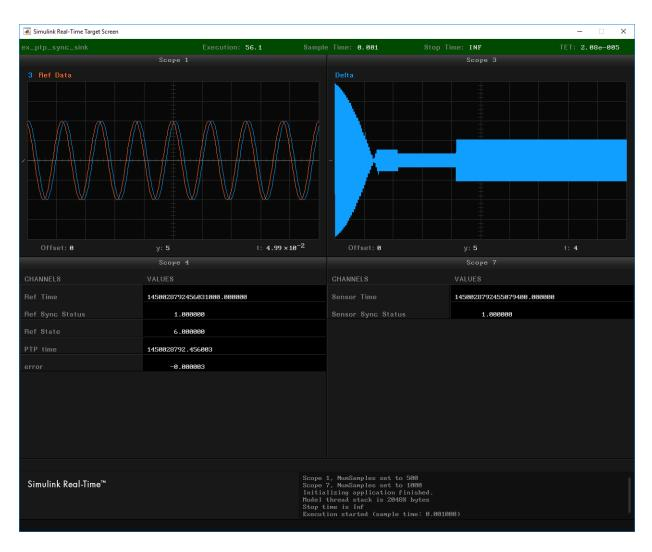
For this example, the sensor and reference Sine Wave blocks are set to the same frequency and amplitude, but start at arbitrary times. The difference in start time causes a phase difference between the sine waves. The phase difference appears on the Delta scope as a waveform that settles to a constant amplitude.
