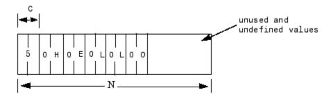
These serial blocks interpret each entry in the vector as a single character. The low-level Send block writes the low-order byte of each entry to the UART. The 16-bit and 32-bit data types allow the embedding of 8-bit data values, including 0. The 8-bit data type is most useful with the ASCII Encode and Decode blocks. The 16-bit and 32-bit data types are most useful for binary data streams.
