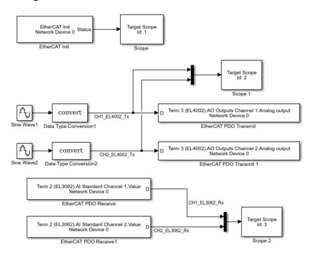
Before configuring the model, carry out the steps in "Configure EtherCAT Network with TwinCAT 3" on page 10-7.
