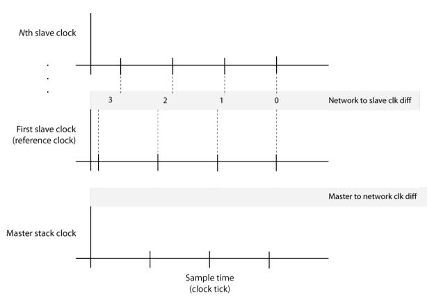
In phase 2, the algorithm shifts the sample time of the master stack running on the target computer to align with the first slave node clock. In that process, the EtherCAT Init block output value MasterToNetworkClkDiff decreases to near zero.
