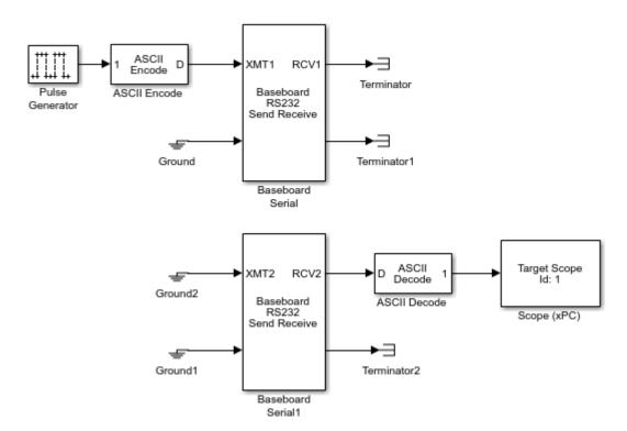
**14** Double-click a Baseboard RS232 Send Receive block. To configure the ports on the target computer for this board, enter values.
