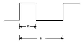
For a base frequency b, this algorithm results in a rectangular output signal of frequency b/n and duty cycle m/n. Because m and n must be integers, it is not possible to provide a continuous range of output frequencies and duty cycles with perfect exactness.
