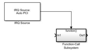
In the setup shown above, the CPU executes the contents of the Function Call-Subsystem whenever IRQ 5 occurs.
