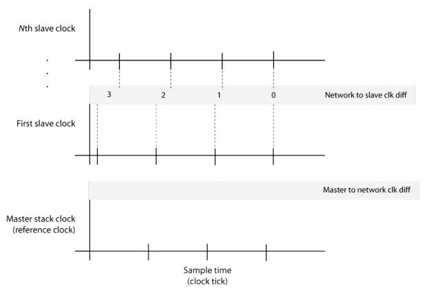
In phase 2, the algorithm shifts the sample time of the first DC-enabled slave node to align with the clock of the master stack. In that process, the value MasterToNetworkClkDiff decreases to near zero. The algorithm shifts the sample time of the other network nodes to stay aligned with the first slave node clock. In that process, the value of NetworkToSlaveClkDiff first increases, then decreases to near zero.
